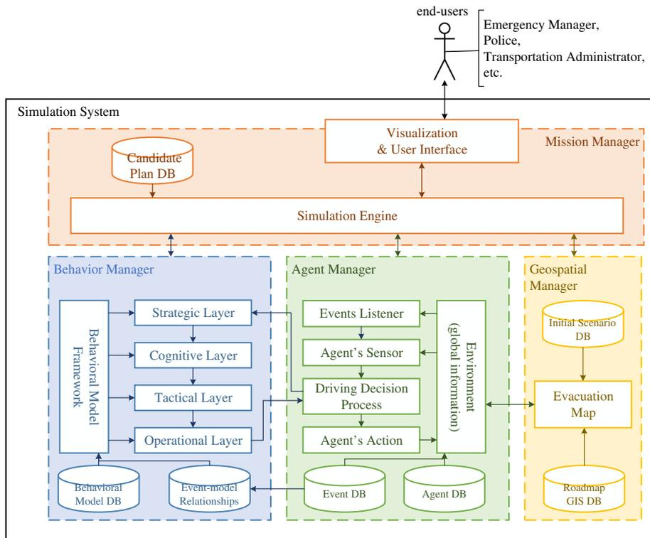
Fig. 1. Components and architecture of the simulation system.
