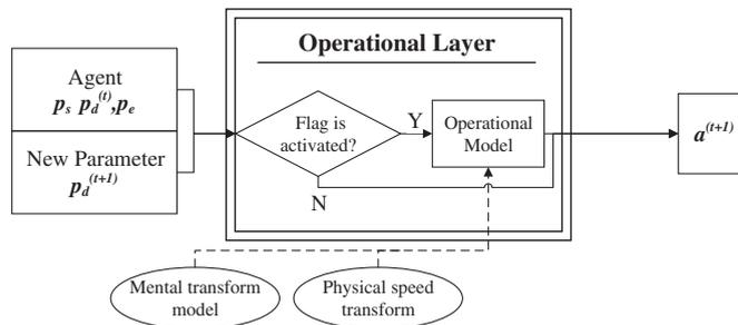
Fig. 7. Flowchart of the Operational Layer.
