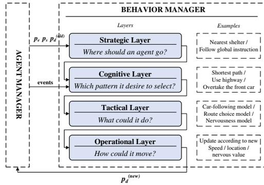
**Fig. 2.** Architecture of the agent-based driving decision process.
